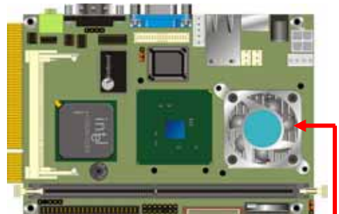
2. Put the cooler on the socket
